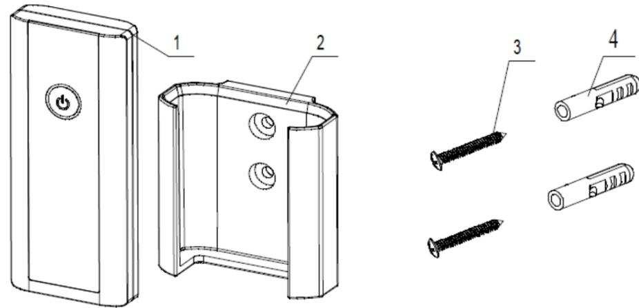
4.1 Drill two holes with diameter 6mm, depth 35mm, and holes distance 16mm. Suggest to install controller outside of the shower enclosure.
